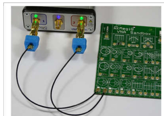
Typical calibration setup on the MegiQ VNA Sandbox
